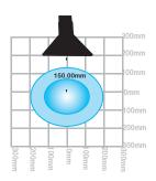
Diagrams above highlight the capture area of the stay put arms when extracting at a flow rate of 60m³/hr (darker shading) and 100m³/hr. These measurements were taken with the arm situated above the working area.
