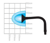
Diagrams above highlight the capture area of the stay put arms when extracting at a flow rate of 60m³/hr (darker shading) and 100m³/hr. These measurements were taken with the arm resting on the work surface.
