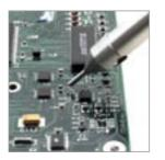
When the precise application of hot air is required, our slim line air pencil (TJ-85 ThermoJet®) is ideal for delivering heat for the installation and removal of chip components, SOTs, and SOICs. Multiple quick-change nozzle sizes are available. The handpiece's slim line, pencil grip design maximizes operator comfort and control. The TJ-85's airflow is actuated with a foot pedal. Ideal for the precise application of hot air for large SMDs down to 0201s.
